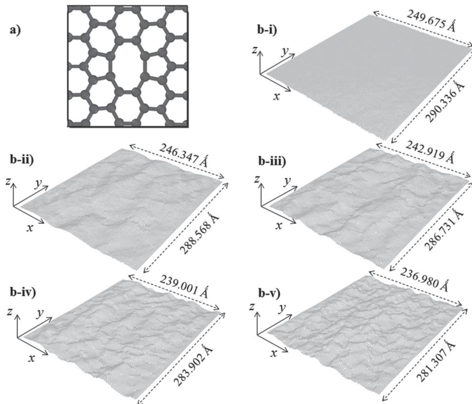
**Figure 1.** a) A representation of a 5–8–5 double vacancy defect in graphene and b) typical images of different systems at increasing defect concentration: i)  $p = 0\%$ , ii)  $p = 0.5\%$ , iii)  $p = 1.0\%$ , iv)  $p = 2.0\%$ , and v)  $p = 3.0\%$ . Note that as the concentration of defects increases, the graphene sheets adopt a more wrinkled conformation thus achieving a shape which resembles that of a wrinkled paper model.
