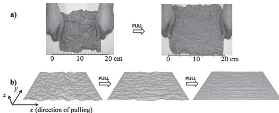
**Figure 2.** a) Typical images of a crumpled sheet of paper at different levels of applied strain and b) typical images of a graphene sheet having 3.0% defects at different levels of applied strain. Note that both systems undergo a de-wrinkling process so as to assume a more planar conformation resulting in an in-plane negative Poisson's ratio.
