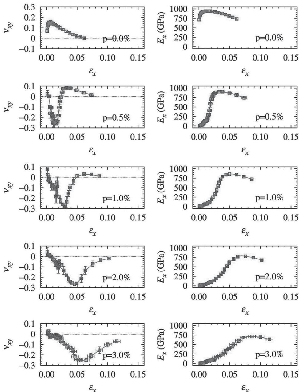
**Figure 3.** The averaged in-plane Poisson's ratios and Young's moduli (calculated from the differential strains) plotted against the engineering strain for stretching in the  $x$ -direction as obtained from the simulations of pristine graphene ( $p = 0.0\%$ ) and the imperfect graphene systems ( $p = 0.5\%$ ,  $1.0\%$ ,  $2.0\%$ , and  $3.0\%$ ).
