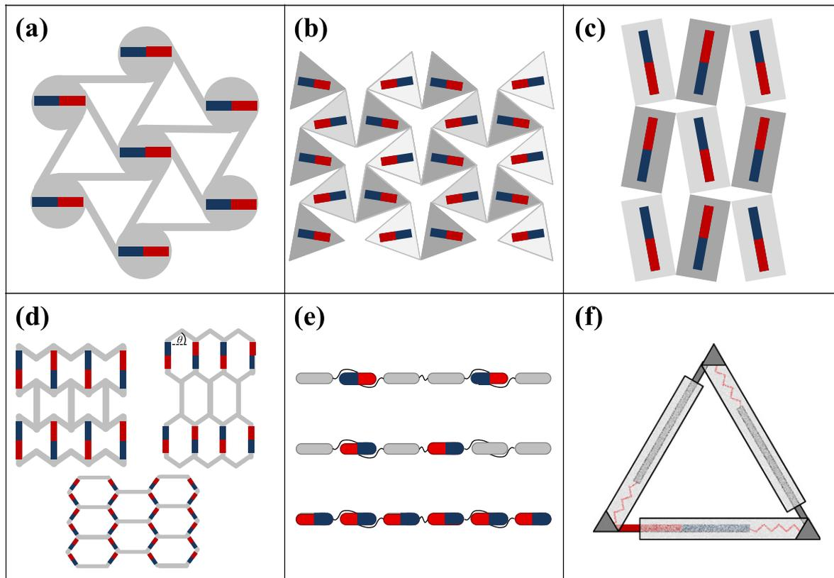
**Figure 1.** Various auxetic structures which lend themselves well to hosting magnetic insertion/s: (a) chirals, (b) rotating rigid triangles, (c) rotating rigid quadrilaterals, (d) honeycombs, (e) liquid crystalline polymers and (f) dilating triangles.
