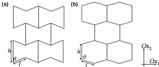
Figure 1. The (a) re-entrant; and (b) non re-entrant hexagonal honeycombs made from rod elements of lengths  $h$  and  $l$  at an angle  $\theta$  to each other. Note that in the EMUDA models, the axes  $Ox_1$  and  $Ox_2$  will be set parallel to the  $Y$  and  $Z$  axes, respectively.
