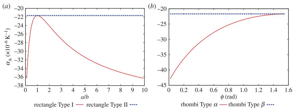
**Figure 2.** (a) Plot of area CTE [ $\times 10^{-6} \text{ K}^{-1}$ ] against  $a/b$  ratio for rectangular-based networks; (b) plot of area CTE [ $\times 10^{-6} \text{ K}^{-1}$ ] against  $\phi$  [rad] for networks composed of rhombi. (Online version in colour.)
