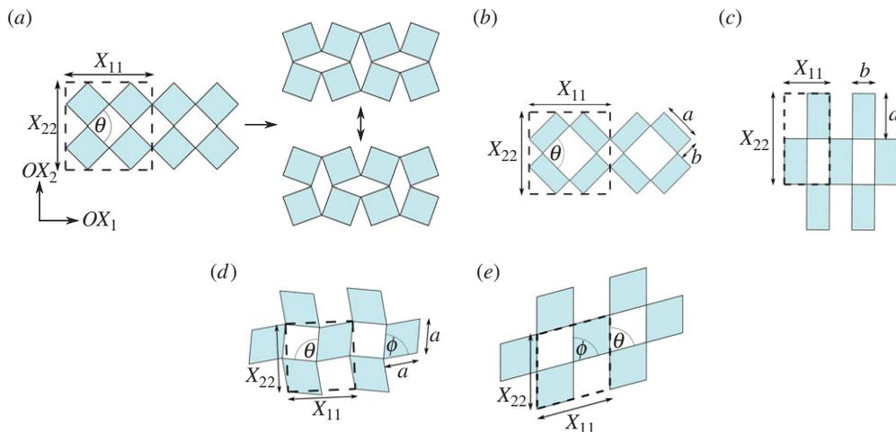
**Figure 1.** Connected networks composed of (a) squares, (b) Type I rectangles, (c) Type II rectangles, (d) Type  $\alpha$  rhombi and (e) Type  $\beta$  rhombi. The respective RUM for the square-based network is also shown in (a); it is assumed that the other geometries follow a similar mode of motion. (Online version in colour.)
