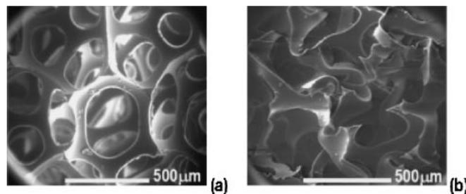
Fig. 1. SEM images of (a) conventional (non auxetic) open-cell polyurethane foams, and (b) auxetic open-cell polyurethane foam.
