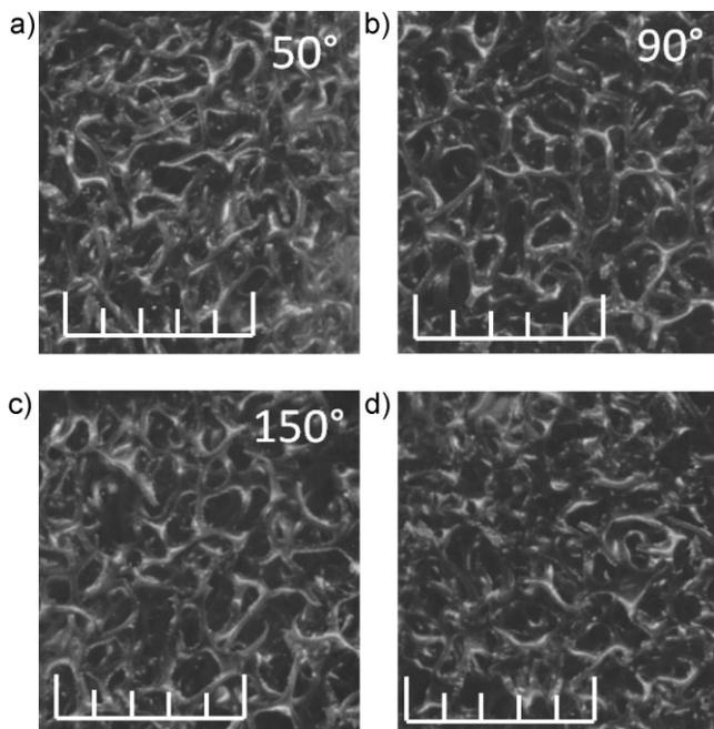
**Figure 4** The microstructure of the auxetic foam when subjected to (a) 50 °C, (b) 90 °C, (c) 150 °C and (d) to the latter temperatures whilst the auxetic foam was in a rigid container of equal dimensions. The scale indicates a distance of 5 mm.
