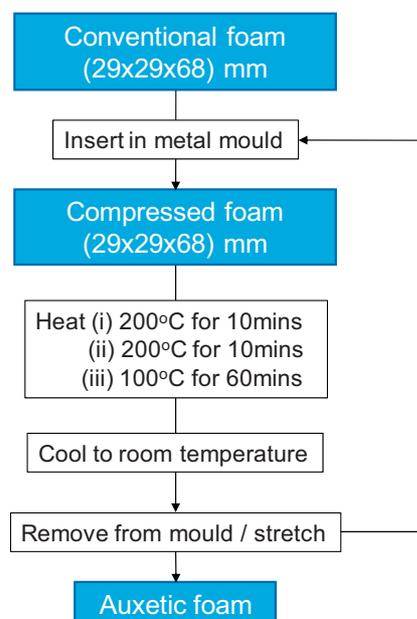
**Figure 1** (online colour at: [www.pss-b.com](http://www.pss-b.com)) Summary of the thermo-mechanical process used to produce the auxetic foams in this work.
