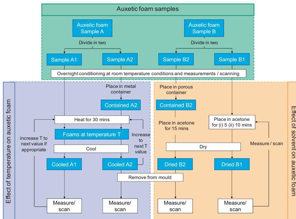
**Figure 3** (online colour at: [www.pss-b.com](http://www.pss-b.com)) A summary for the procedure used in testing the effect of temperature and solvent on auxetic foams.
