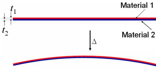
**Figure 1.** The effect of heat on a bi-material strip made from materials “1” and “2” where the materials have different thermal expansion coefficients  $\alpha_1$  and  $\alpha_2$  where  $\alpha_1 > \alpha_2$ . Here we are proposing that the same effect may be achieved if the strip is subjected to a change in the external pressure provided that the Young’s moduli and/or Poisson’s ratio of material “1” are different from those of material “2”.
