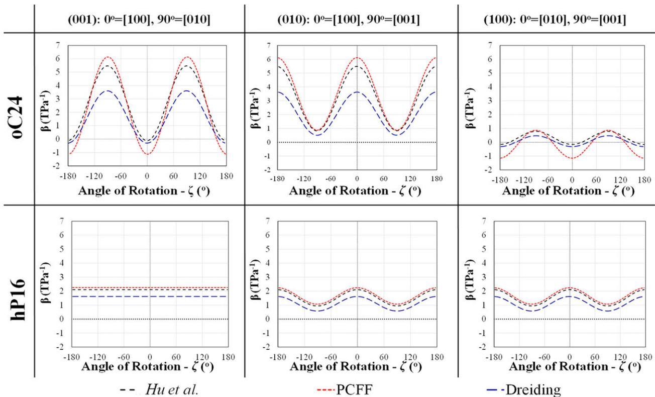
**Figure 4** Calculated off-axis linear compressibility plots for the hP16 and oC24 networks as simulated using the Dreiding and PCFF forcefield compared with the results obtained by Hu et al., using *ab initio* simulations [39].
