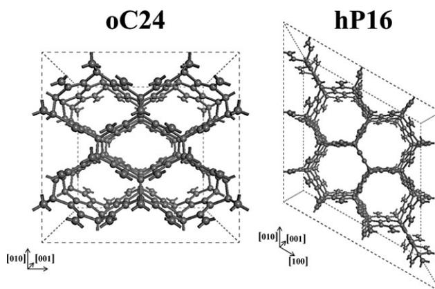
**Figure 2** Perspective views of (001) planes of the hP16 and oC24 networks constructed from the coordinates as simulated by Hu et al. [39].
