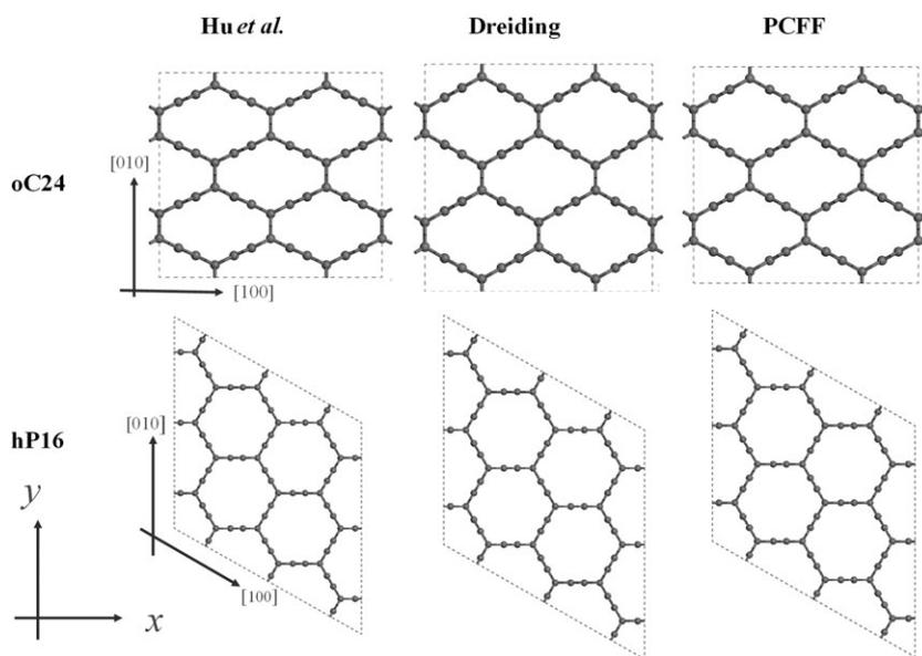
**Figure 3** Projections of (001) planes of the hP16 and oC24 networks simulated using the Dreiding and PCFF force-fields and those simulated by Hu et al. [39].
