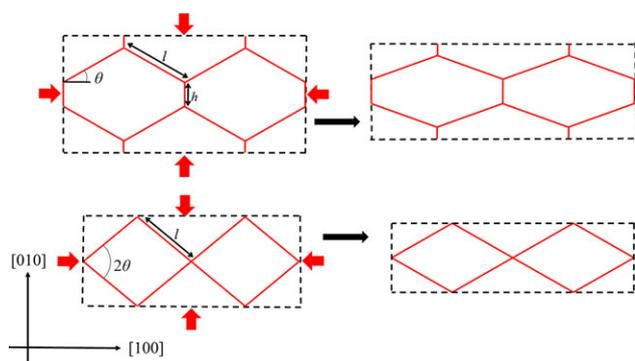
**Figure 1** Negative linear compressibility from 2D non-re-entrant honeycomb systems and the particular case of 2D wine-rack-like systems. Note that in both cases the maximum NLC behavior is measured in the [100] direction [32].
