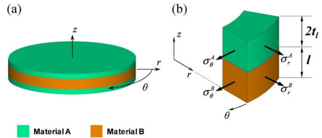
**Figure 3** The system modeled and the dimensions used: (a) cylindrical coordinate system and (b) a simplified elemental diagram showing the stresses on each material in the  $r\theta$ -plane where material A has the overall length ( $2t_l$ ) of both the top and bottom layers in the figure on the right.
