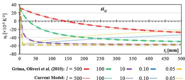
**Figure 5** Comparison of the CTE in the axial direction ( $\alpha_l$ ) between the model presented by Grima et al. [23] and the one presented here. Note that for systems where  $t_l$  is small, which are the most interesting systems from a NTE point of view, the deviations are very significant, thus highlighting the importance of the current model.
