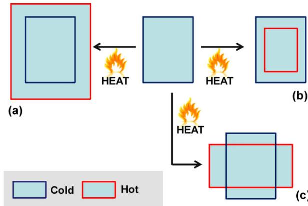
**Figure 1** System showing (a) isotropic positive thermal expansion, (b) isotropic negative thermal expansion (NTE), and (c) anisotropic thermal expansion with conventional thermal expansion in the horizontal direction and NTE in the vertical direction.
