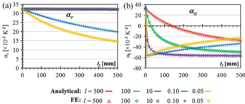
**Figure 4** Comparison of the CTE in the (a) radial and (b) axial directions of FE results presented elsewhere [25] with the analytical models derived here. Note that the FE data relates to the system in Fig. 2a for the special case when  $t = 0$ , i.e., the structure similar to the one shown in Fig. 3a.
