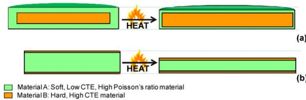
**Figure 2** (a) The concept of achieving NTE from a coin-shaped, high-CTE hard inclusion inside a soft low-CTE high Poisson's ratio matrix [25]. (b) The concept of achieving NTE from a sandwich, having high-CTE hard surrounding a soft low-CTE high Poisson's ratio matrix [23].
