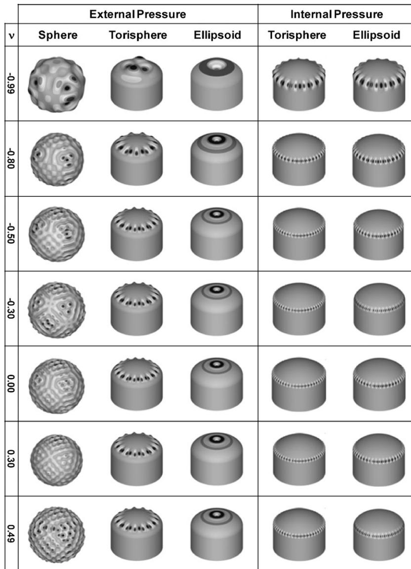
**Figure 6** Contours showing the transverse displacements of the first eigenmode of some shells analysed.
