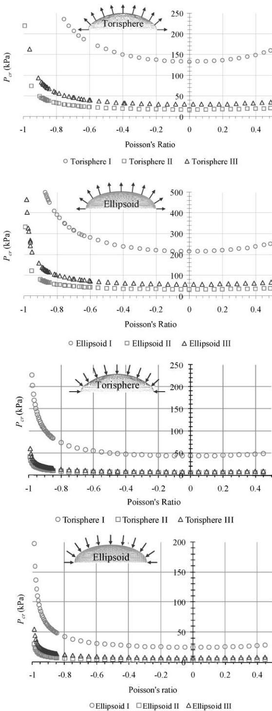
**Figure 4** Plots showing the effect of the Poisson's ratio on the critical buckling pressure of the torispherical and ellipsoidal heads applied according to the diagrams.
