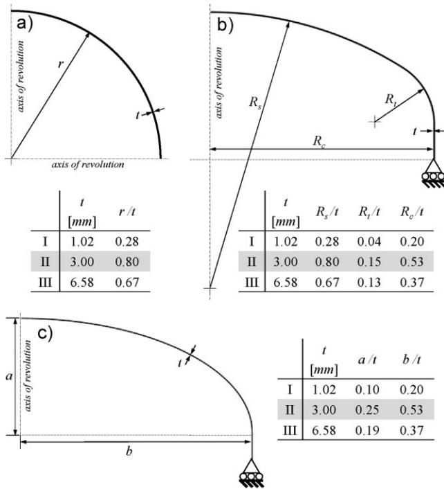
**Figure 1** Dimensions of the (a) spheres, (b) torispheres and (c) ellipsoids analysed.
