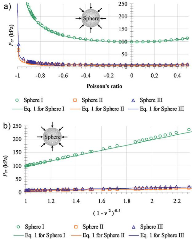
**Figure 2** (online colour at: [www.pss-b.com](http://www.pss-b.com)) Plots of the variation of the critical buckling pressure  $P_{cr}$  with (a) the Poisson's ratio  $\nu$  and (b) the  $(1 - \nu^2)^{-1/2}$  fraction together with a linear regression of the form  $y = mx + c$ .
