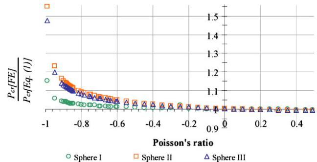
**Figure 3** (online colour at: [www.pss-b.com](http://www.pss-b.com)) Plots of the ratio between the critical buckling pressure given by the FE  $P_{cr}[FE]$  and the theoretical one  $P_{cr}[Eq. (1)]$ .
