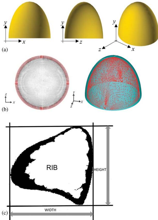
**Fig. 2.** (a) Views and (b) boundary and loading conditions for the ellipsoid FEA chest model. (c) Diagram showing measurements performed on the ribs. Height was measured tangential to the plane of the curvature of the ribs in the mid-axillary line. [Color figure can be viewed in the online issue, which is available at [wileyonlinelibrary.com](http://wileyonlinelibrary.com).]
