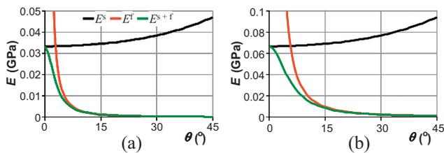
**Figure 5** (online colour at: [www.pss-b.com](http://www.pss-b.com)) Plots showing the variation of the Young's modulus for stretching, flexing and combined stretching and flexing as a function of  $\theta$ . For these particular cases,  $l = 10$ ,  $h = 15$ ,  $E_s = 1$  GPa and (a)  $t = 0.5$ , (b)  $t = 1$ .
