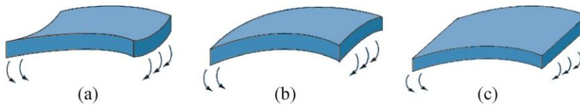
**Figure 6** (online colour at: [www.pss-b.com](http://www.pss-b.com)) Bending in (a) conventional, (b) auxetic and (c) zero Poisson's ratio material. The edges along which the bending stress is applied deform in a different manner in each case. In conventional materials the edge curves upward to form a saddle shape (a), in auxetic materials it curves downwards to form a dome shape (b) while in zero Poisson's ratio materials it remains straight (c).
