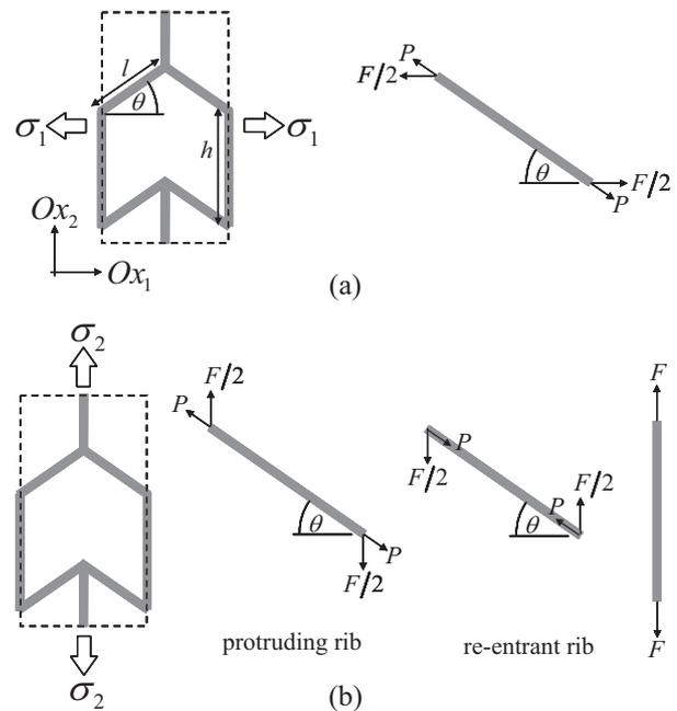
**Figure 2** Force components acting along the inclined ribs when the semi re-entrant honeycomb deforms through stretching for loading in the (a)  $Ox_1$  and (b)  $Ox_2$  direction.
