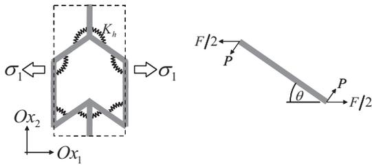
**Figure 3** Force components acting perpendicular to the inclined ribs when the semi re-entrant honeycomb deforms through hinging when loading in the  $Ox_1$ .
