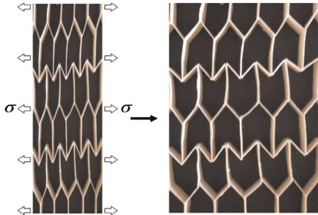
**Figure 4** (online colour at: [www.pss-b.com](http://www.pss-b.com)) Deformation in a semi re-entrant honeycomb made of cardboard, showing that in such a honeycomb deformation occurs mainly through hinging.
