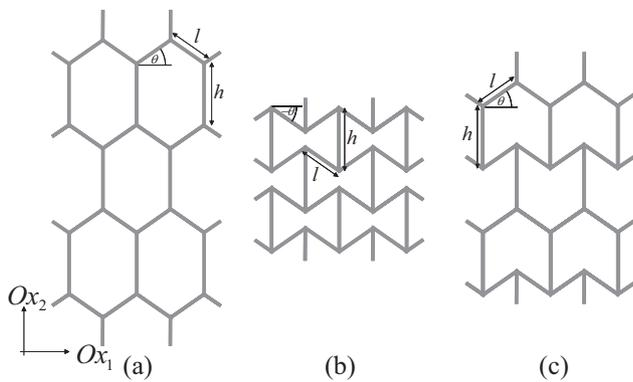
**Figure 1** Geometry of the (a) conventional, (b) re-entrant honeycomb and (c) the semi re-entrant honeycomb.
